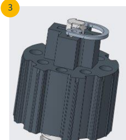
Push the C-Ring down to secure the drive wheel.
