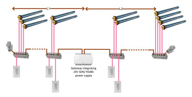
L1: the current needed by powered devices is 240mA. Chart -> max. possible 500 m.
