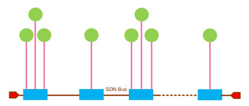
SDN bus: The maximum length cannot exceed 1000 m and refers to the controller documentation. Junction: **passive** must be used.
