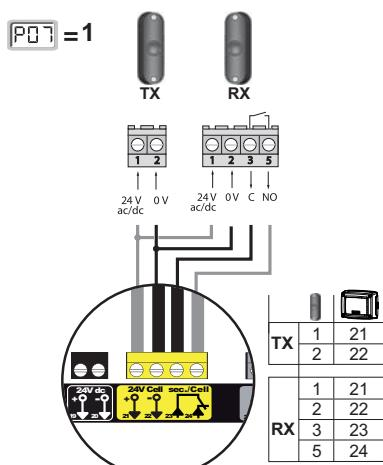
**Photoelectric cells - with autotest**
