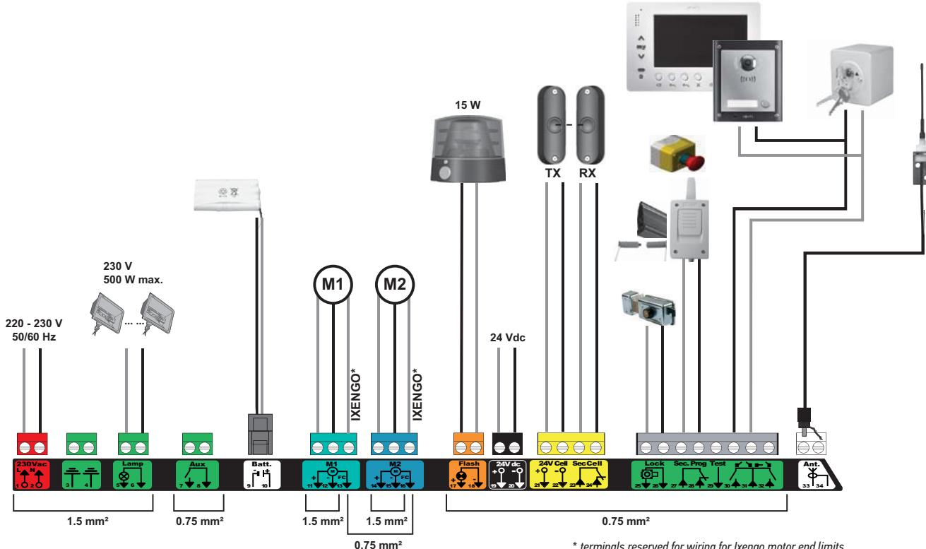
**Photoelectric cells - without autotest**
