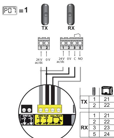
**Foto-elektrische cellen - met zelftest**
