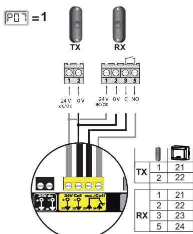
**Fotoseller - otomatik test var**
