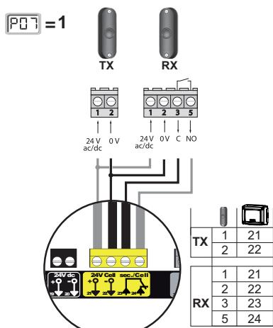
**Photoelectric cells - with autotest**
