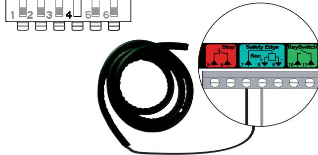
**!** If a wired safety edge replaces a radio safety edge, the radio safety edge transmitter must be cleared (see section 12) to ensure the wired safety edge is taken into account.
