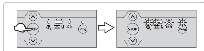
When holiday mode is active, each time a locked control (programming interface or remote control) is pressed, indicator lights 1, 2, 4 and Prog start flashing for 2 seconds.
