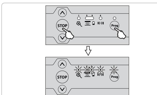
To lock the programming buttons, repeat the locking procedure described above.
