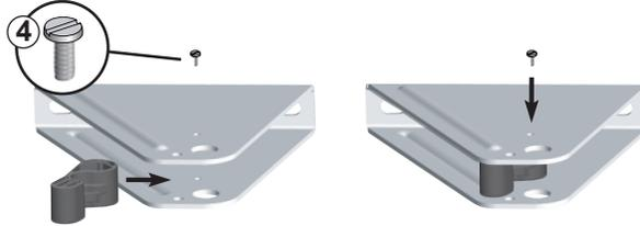
**!** The direction of fitting indicated in the diagram must be respected for correct operation of the unlocking mechanism. Do not fit the screw from below.
