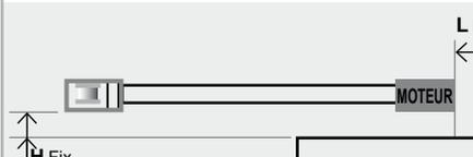
$$L \text{ Fix} = \frac{L \text{ Vantail} - L \text{ Ouverture}}{2} - 46$$
