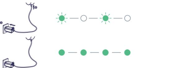
The battery must be fully charged before first use.
